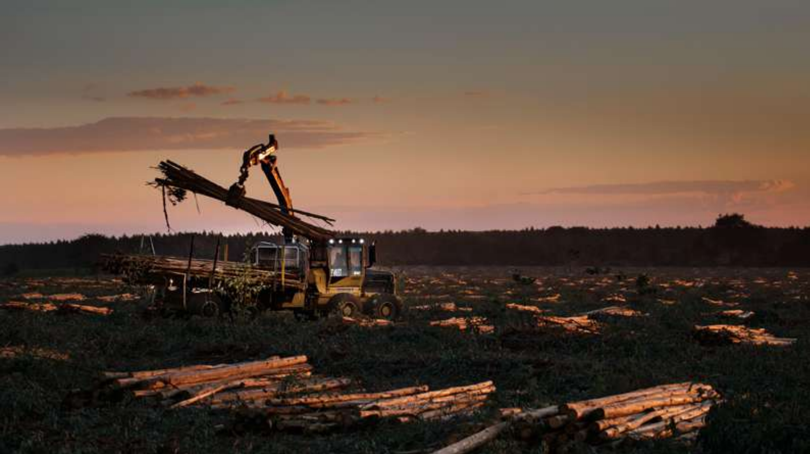
Forwarder machine stacking eucalyptus logs after harvest, in Mato Grosso do Sul state. Photo: Araquém Alcântara
